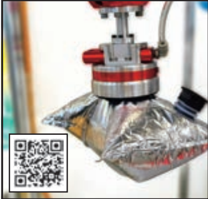
SGR Conveyance of bags of liquid by vacuum hand specially designed for bags
