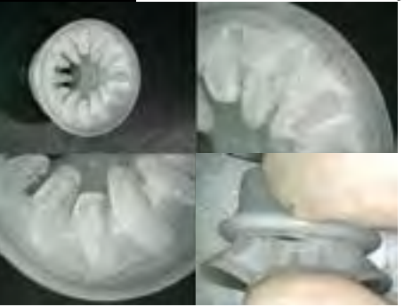
PYKG-20-S5 Unusable after 520,000 Cycles (Bellows Tear)
