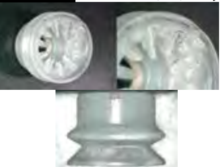
PYKG-15-S5 Usable after 1,000,000 Cycles (Wear Observed)
