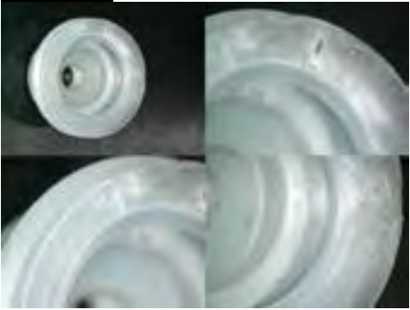
PJG-20-S Unusable after 140,000 Cycles (Lip Puncture)
